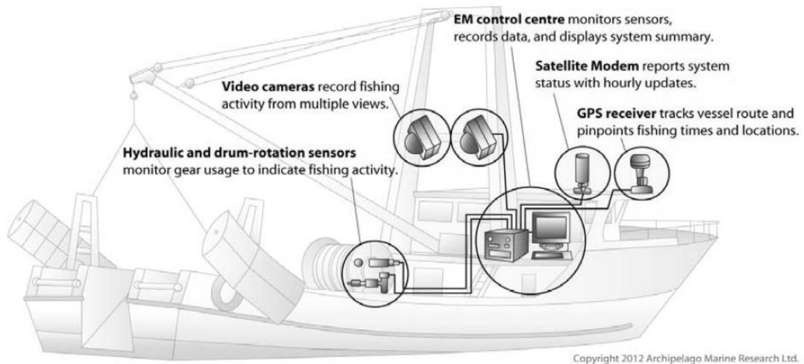
**Figure 3 Schematic diagram of EM equipment. Source (Piasente, et al., 2012)**
