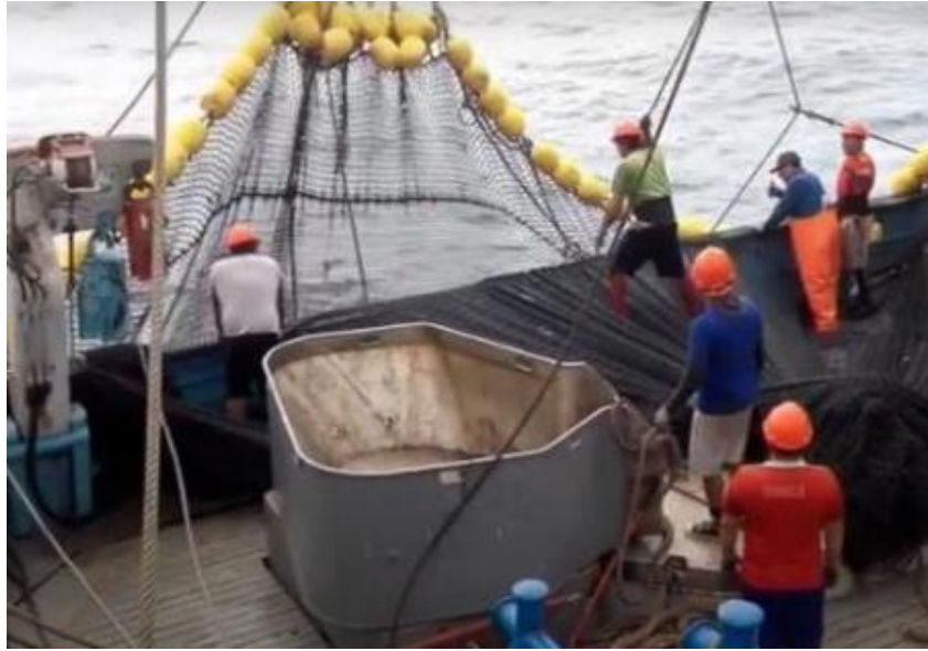
Figure 1. Small sized hopper with high walls, which prevents effective bycatch detection and release during brailing.
