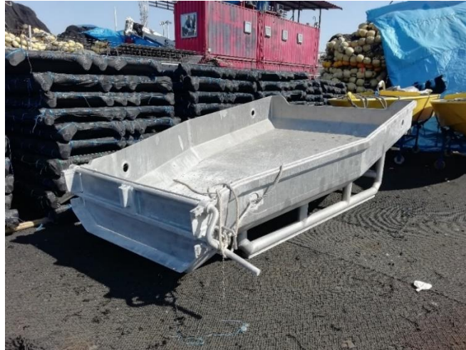
Figure 4. Hopper from a vessel studied stored at port during unloading.
