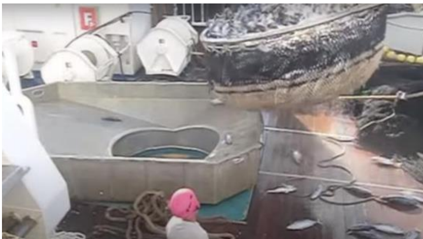
Figure 2. Large hopper tray lacking a stoppage door to prevent bycatch going down to quickly into the unloading hatch opening to the lower deck.
