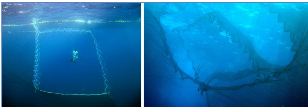
Figure 3. The closed release panel and the panel opening immediately after the zipper line has been pulled
