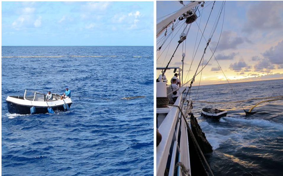
Figure 11. Workboat towing a drifting FAD (left) and exiting the net after pursing is complete (right).
