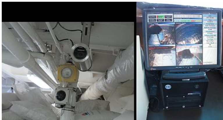
Figure 8. Archipelago system camera (bottom left) and control box/monitor onboard the Cape Finisterre.
