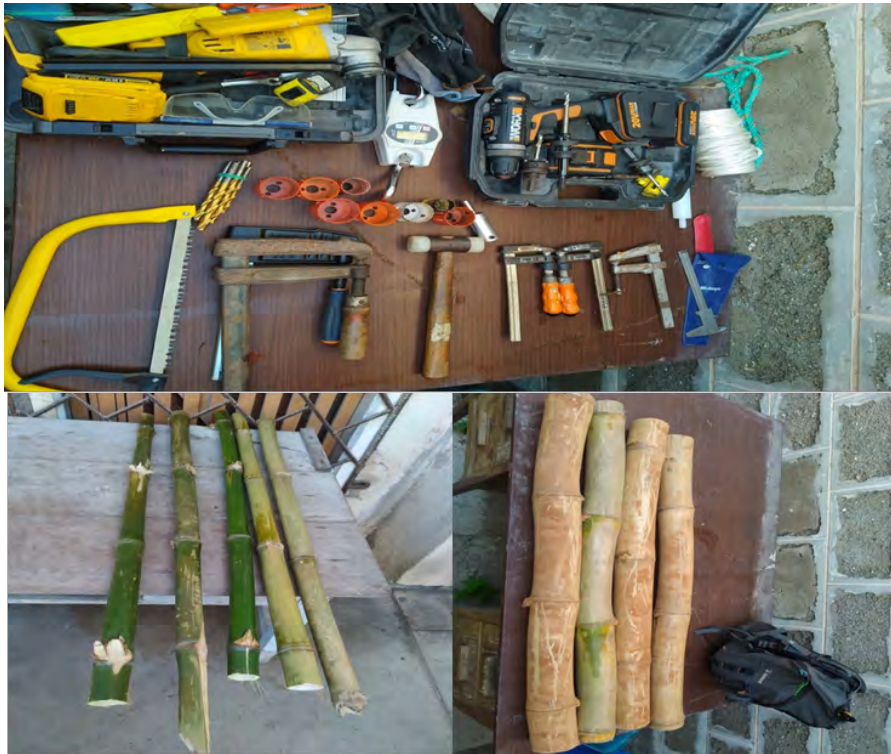
Figure 1. Tools and bamboo canes needed to build the biodegradable FAD.
