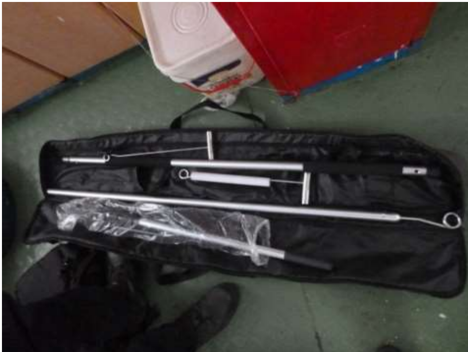
Figure 9. Fishing vessels are required to carry sea turtle bycatch mitigation devices such as dip nets, line cutters and de-hookers. This vessel could be considered compliant as the gear is present, but it is clear that the gear has not been used and is not stored in a location that facilitates its use. Source: AFMA
