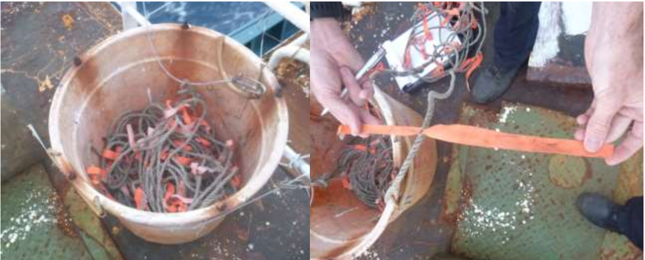
Figure 11. Op Nasse 2018 observed tori line made from rope and flagging tape. This tori line did not meet CMM specifications. Source: AFMA
