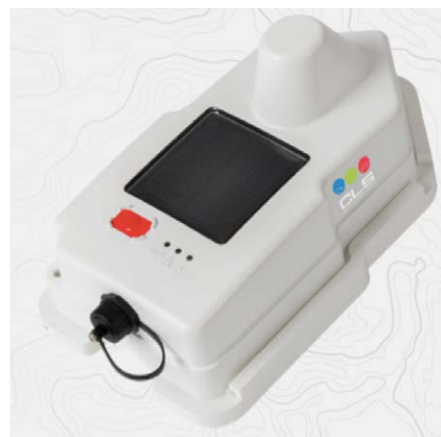
Figure 18: CLS's hybrid satellite transponder.
