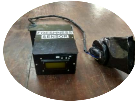
Figure 16: ICAR – the Central Institute of Fisheries Technology's handheld freshness sensor.
