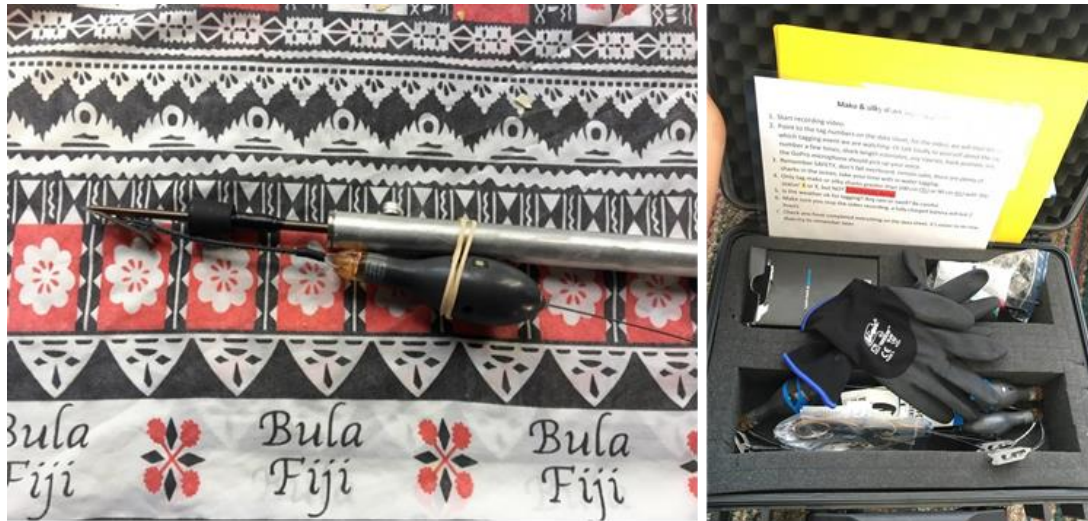
Figure B1: Tag attached to the tag pole (left) and tagging kit (right). Image: Caroline Sanchez (SPC)
