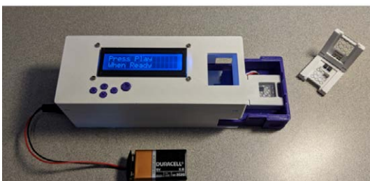
Figure 11: Conservation X Lab's hand held DNA scanner.
