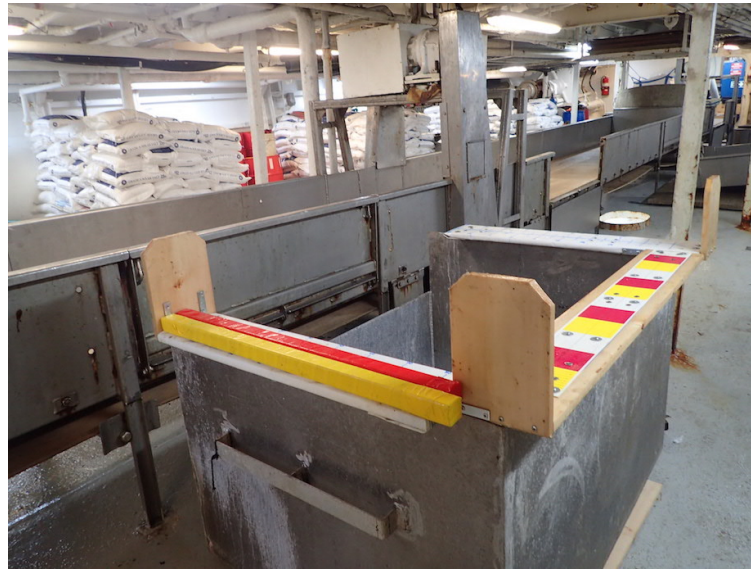
Figure 7. Spill sample bin with measuring boards in place adjacent to the conveyor belt spill door.
