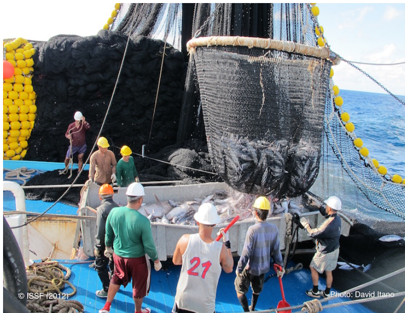
Figure 1. Brailing catch into a sorting hopper prior to release to the wet deck and storage wells.
