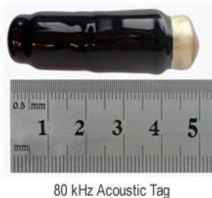
Figure 6: HTI Sonar 980 series acoustic tag for marine uses (source: HTI Sonar)
