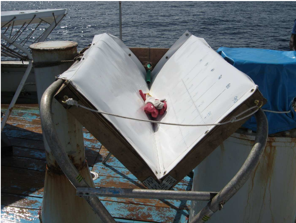
Figure 1. V-shape tagging cradle re-designed for archival tagging.
