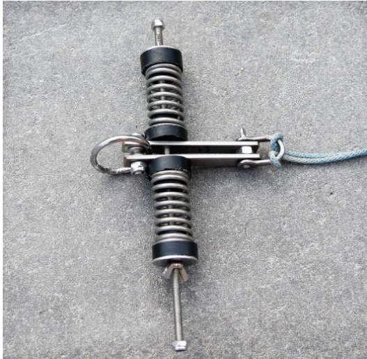
Figure 7: Tension release developed during the course of the project. The bird-scaring line is attached to the ring and the blue rope to the tori pole. As the wing nuts are tightened more pressure is exerted on the two arms, making it harder to pull the ring out.
