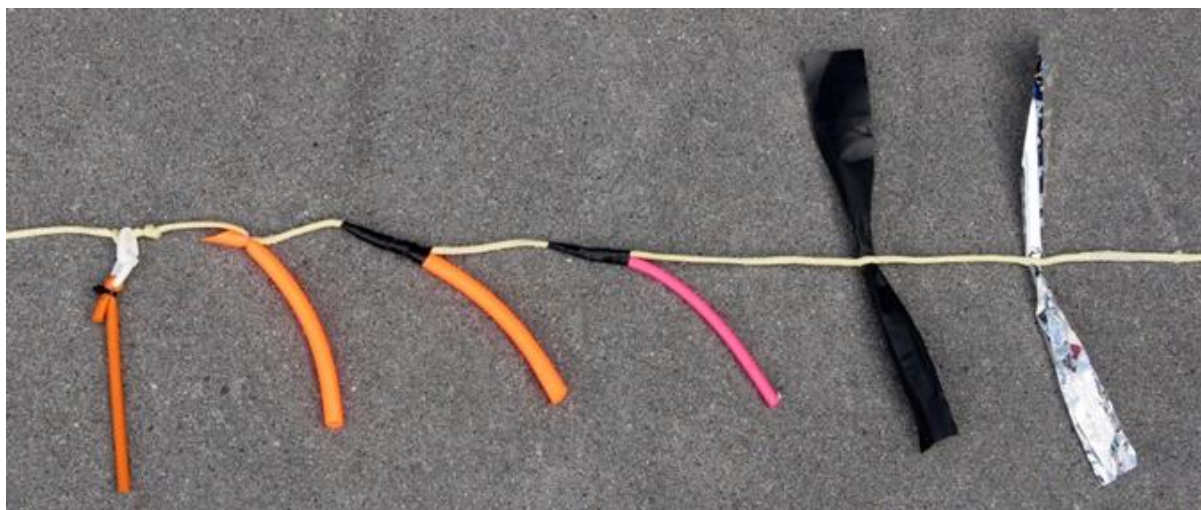
Figure 3: Bird-scaring line backbone, streamer materials and streamer attachment.
