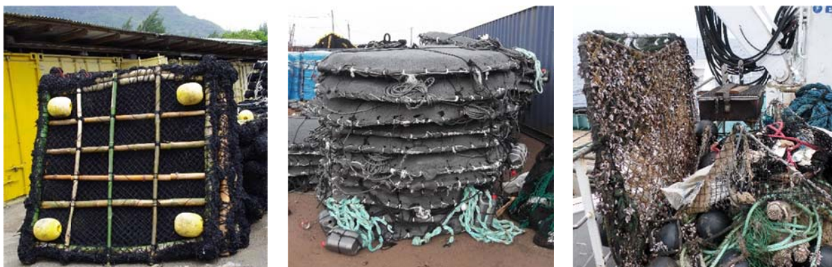
Figure 3. Examples of different dFAD designs and construction materials used in the Indian and Atlantic Oceans. Materials used on the frame include bamboo (left), plastic tubing (middle) and metal tubing (right). Photos: E. Chassot – IRD; KR-C Kouakou - IRD/ORTHONGEL; Anon – IRD.
