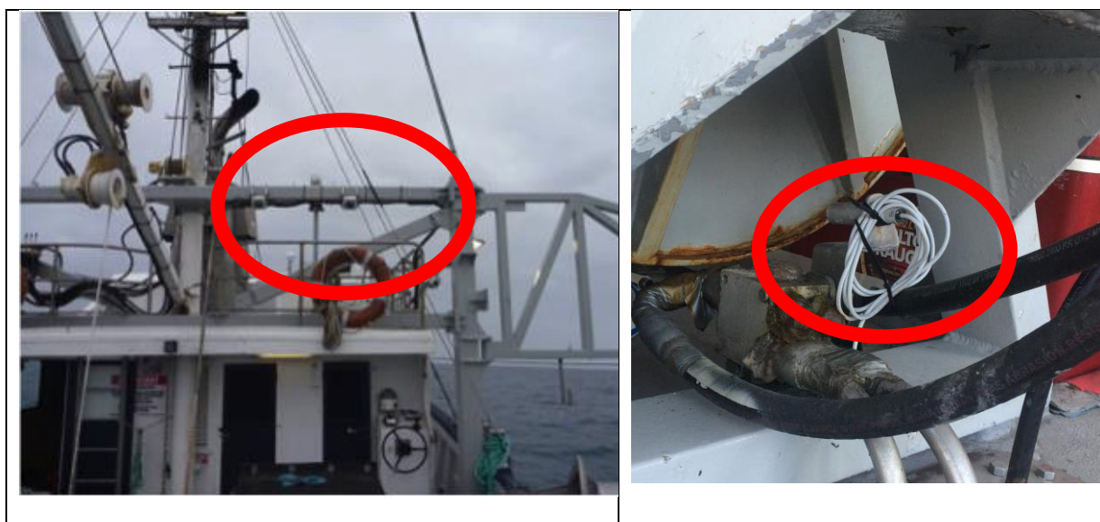
Photo 2: Positioning of (a) cameras and (b) motion sensors
