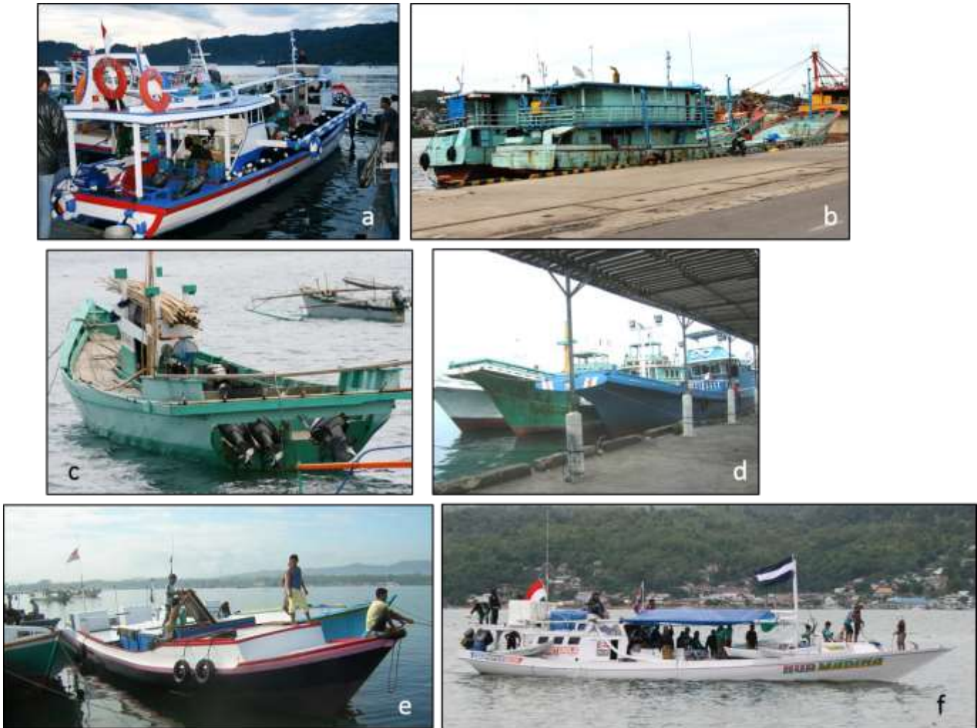
Figure 7. Examples of Indonesian vessel types that fish on FADs: (a) Mini purse-seine ( pajeko ), < 30 GT, at PPP Sodohoa; (b) larger purse-seine ( pukat cincin ), > 30 GT, at PPS Kendari; (c) small pole and line ( funae ) in Belang, North Sulawesi; (d) pole and line, >50 GT, in Sorong; (e) hand-line/troll-line ( penongkol ) at PPP Sodohoa; and (f) hand-line/troll-line ‘mother-ship’ carrying several small catcher boats ( sampan ) in Kendari (Photos: Proctor).
