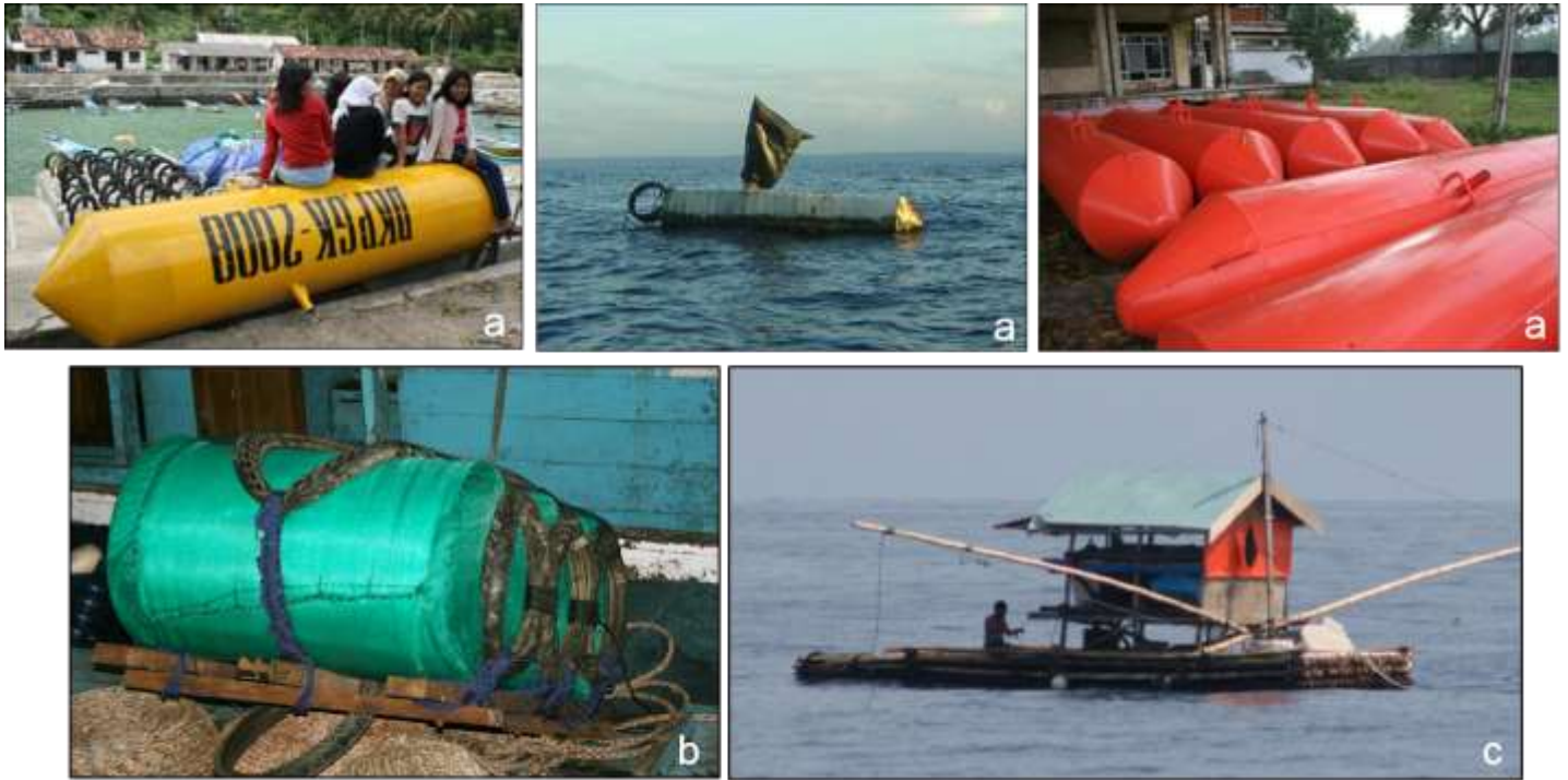
Figure 3. Various types of anchored FAD floats in Indonesia (a) steel ponton , (b) styrene foam gabus , and (c) bamboo raft with rakit (photos: Proctor)
