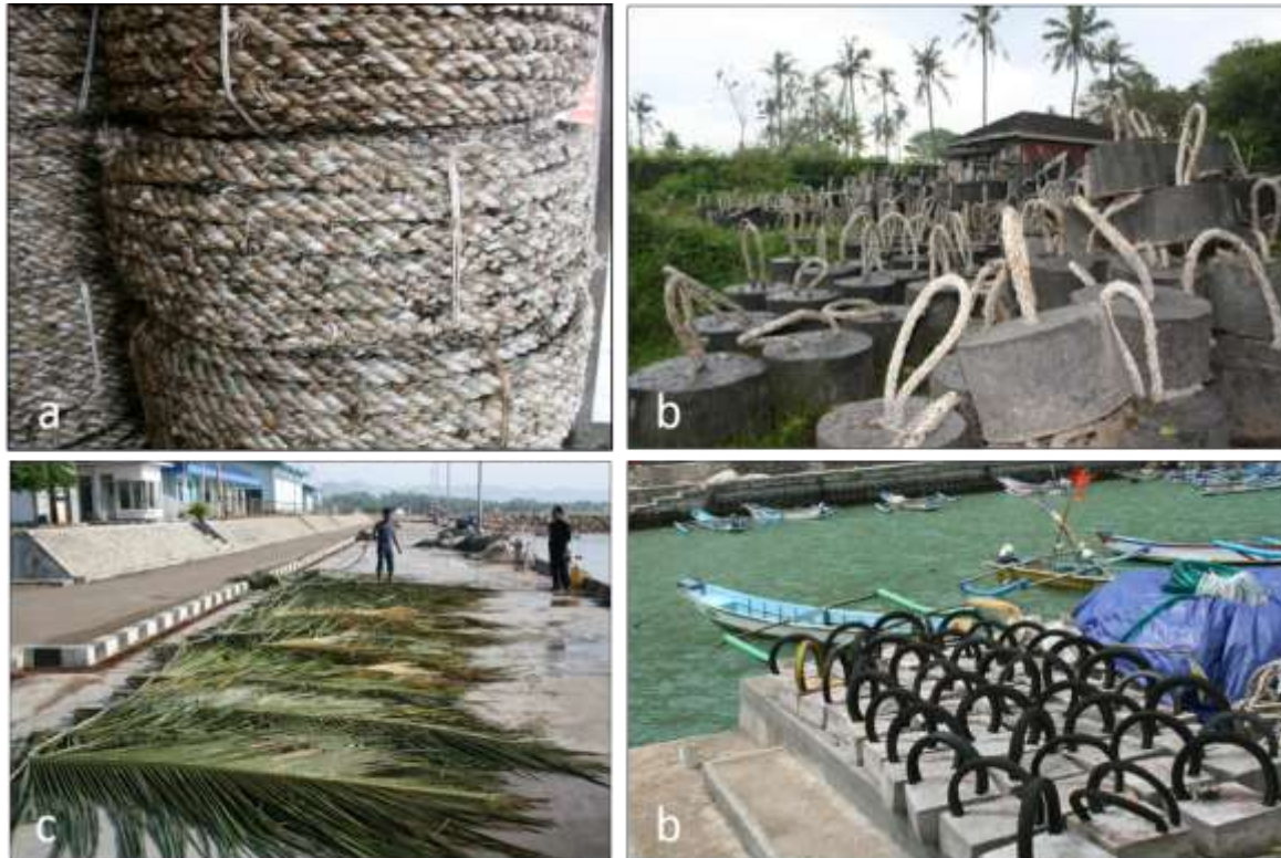
Figure 4. Examples of components for Indonesian anchored FADs: (a) coils of rope used for FAD mainline, (b) 60-80 kg cement weights which are linked together to form the FAD anchor, and (c) coconut palm branches attached to mainline as subsurface attractor (Photos: Proctor).
