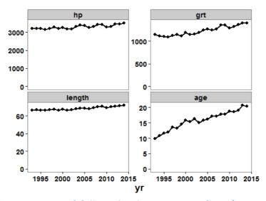
Figure 5. Vessel characteristics of fully utilized purse seine fleet (147 vessels), average, hp=horse power, grt=gross registered tonnage, length=length of vessel (m), and age.
