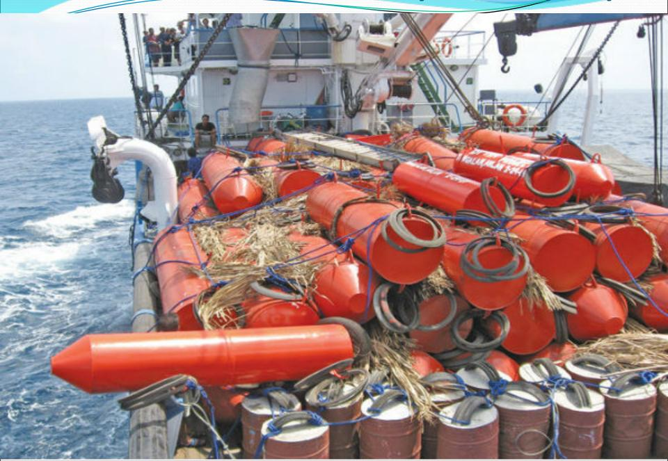
WHF Radio Buoys on drifting FADs, historically limited numbers, tracked within 60 nm radius of vessel, and no indication of what was under each.
