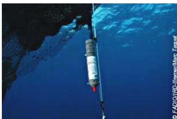
Figure 13 Drifting FAD with detection / acoustic equipment deployed. (Image from http://www.fadio.ird.fr/ )
