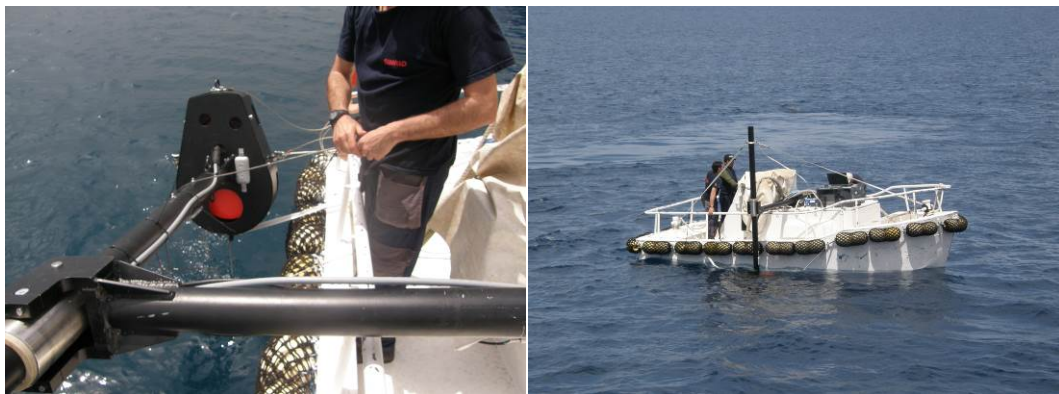
Figure 4. Scientific echo-sounders installed on the work boat ("panguita").
