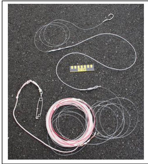
Figure 45. Double weight system on a Japanese tuna branch line. The white section (with scale) is the inelastic section with weights at each end. (Photo credit: E. Melvin)
