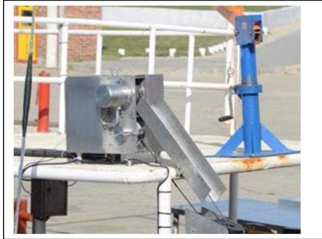
Figure 42. The underwater setting capsule in situ on a vessel in Uruguay (Photo credit: G. Robertson).
