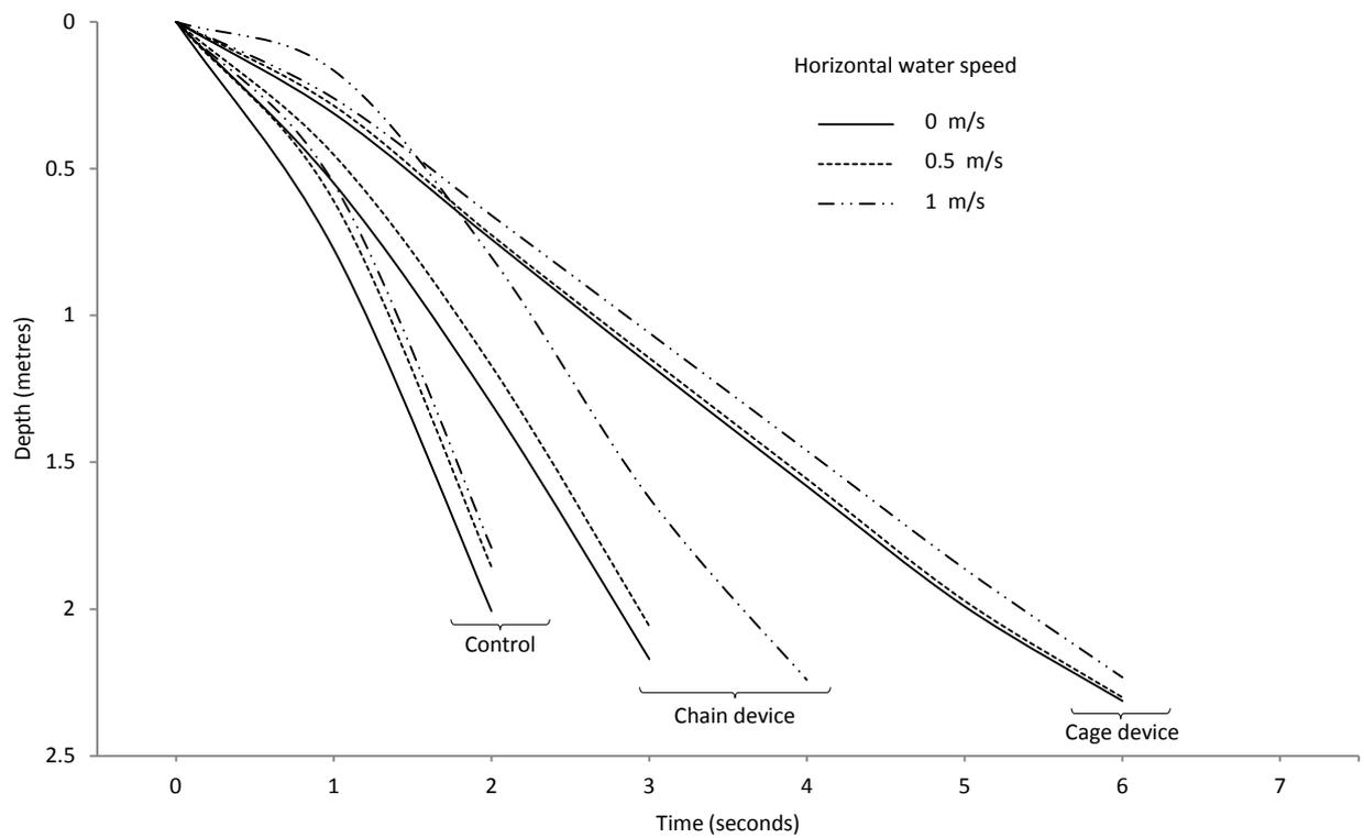
Figure 4 Summary of sink rate experiment in 2.5 m deep CWC, to determine the effect of ‘treatment’ branchlines (i.e. with a *Cage Device* or *Chain Device* attached) and ‘control’ branchlines (i.e. without a device attached) on sink rate during setting, at three horizontal waters speeds.
