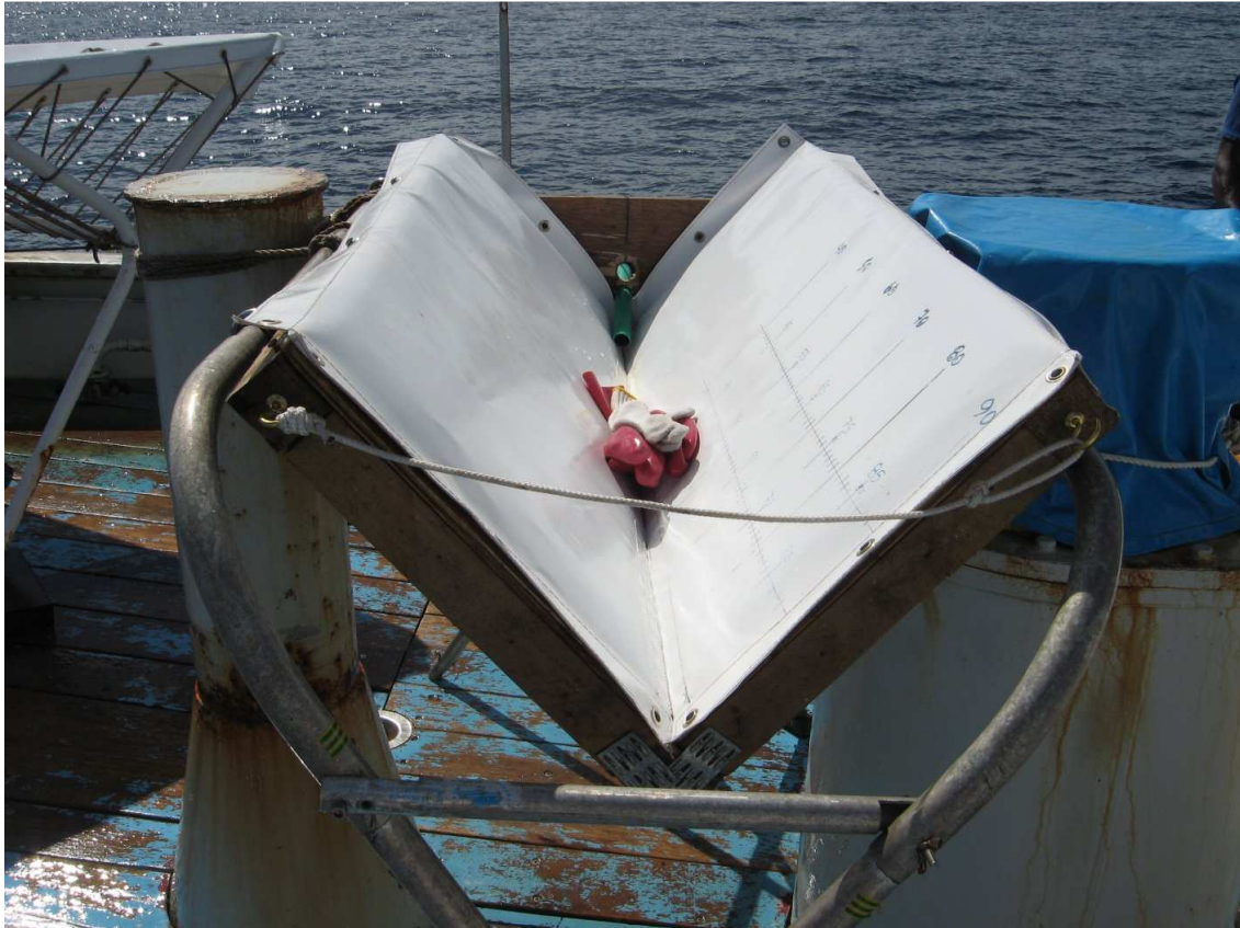
Picture 2. V-shape tagging cradle re-designed for archival tagging.
