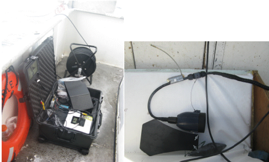
Figure 1. SPLASHCAM video system with viewing/recording gear (left) and camera head (right) rigged prior to deployment
