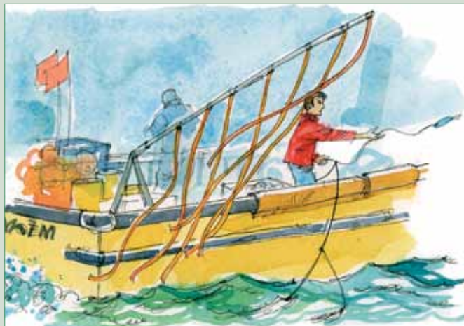
Figure 1. Casting baited hooks forward and close to the hull of the vessel allow baits to start sinking before passing the stern of the vessel.
