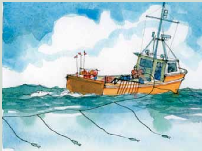
Figure 2. Side-setting with a bird curtain in use.
