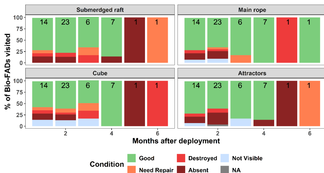
Figure 12. DFAD state with time at sea of the different components of the 52 jelly-FADs visited with condition recorded. Number at the top of each bar corresponds to the number of dFADs visited that month. Some jelly-FADs did not present any attractors, corresponding to a condition recorded as “NA”.
