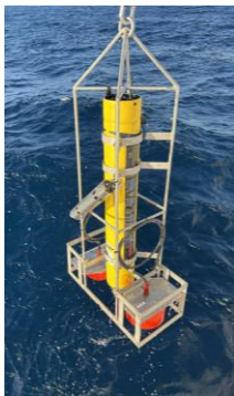
Fig. 6. The profiler WBAT in its frame, equipped with 2 transducers (38 and 120 kHz) and a depth sensor (TDR).
