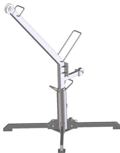
Figure 7. Portable crane that could help dFAD recovery from small vessels (Jefferson Murua, personal communication).
