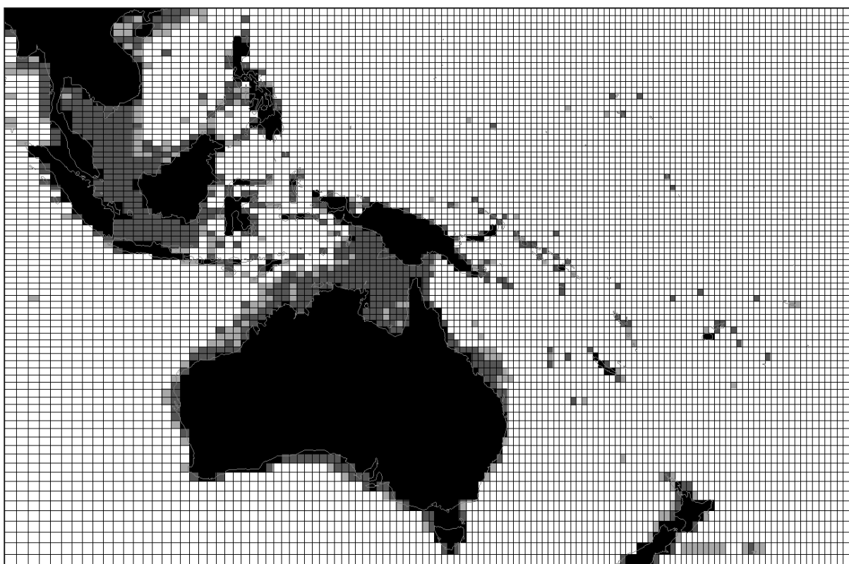
Figure 1: One-dimensional grid stretching in WCPO region and three-layer mask generated by GMB. Land mask is build for 0-100m (grey rectangles), 100-400m (light grey) and deeper 400m (white) layers. The smallest grid resolution is 0.5^\circ .
