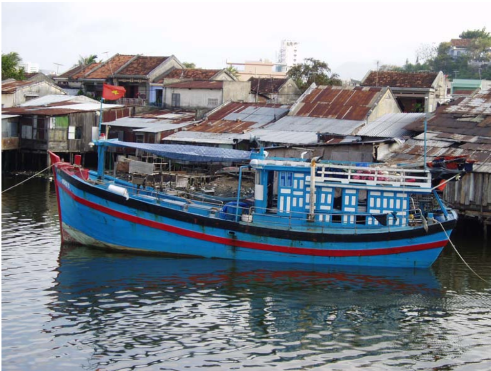
Medium longliner in Nha Trang port. Note line hauler on SB side for'ard and line shooter on stern
