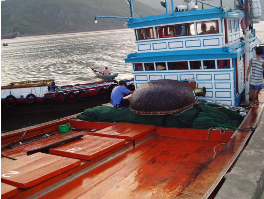
Foredeck of purse seiner in Quy Nhon port, Binh Dinh Province; circular object on covered net is dinghy (coracle); note capstan winch for hauling, and four storage holds.
