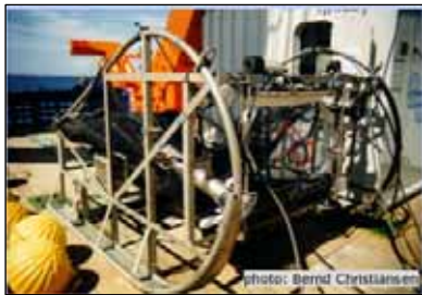
Epibenthic sledge, equipped with additional video and still cameras Bernd Christiansen, Universitat Hamburg 32
