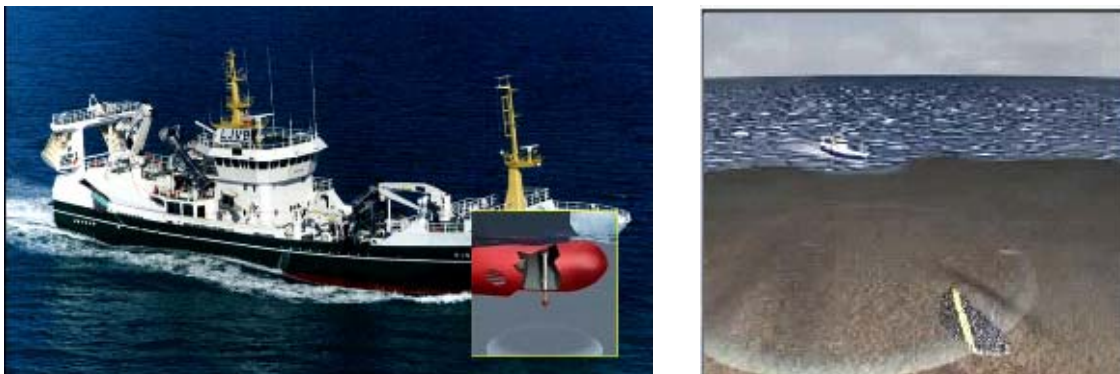
Figure 4a and 4b. Site of omnidirectional sonar on board a fishing vessel: the sonar is generally located in the prow of the vessel (a). Example of fish school detection with the aid of omnidirectional type sonar (b).
