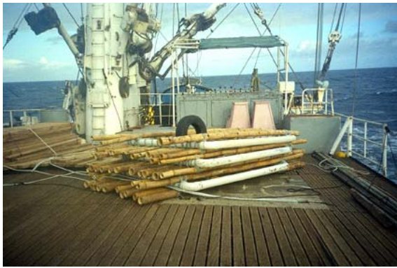
Figure 7. Bamboo anchored FAD rafts used in the Solomon Islands and Fiji to support purse seine operations (photos Brogan, Itano)
