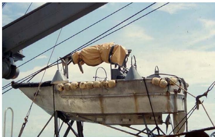
Figure 31. Generator equipped light boat used to aggregate baitfish and tuna on anchored FADs (photo Itano)
