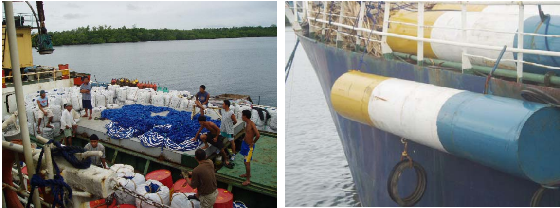
Figure 32. Ranger vessel loaded with FAD mooring lines and an AFAD float ready for deployment (photos Fukofuka)
