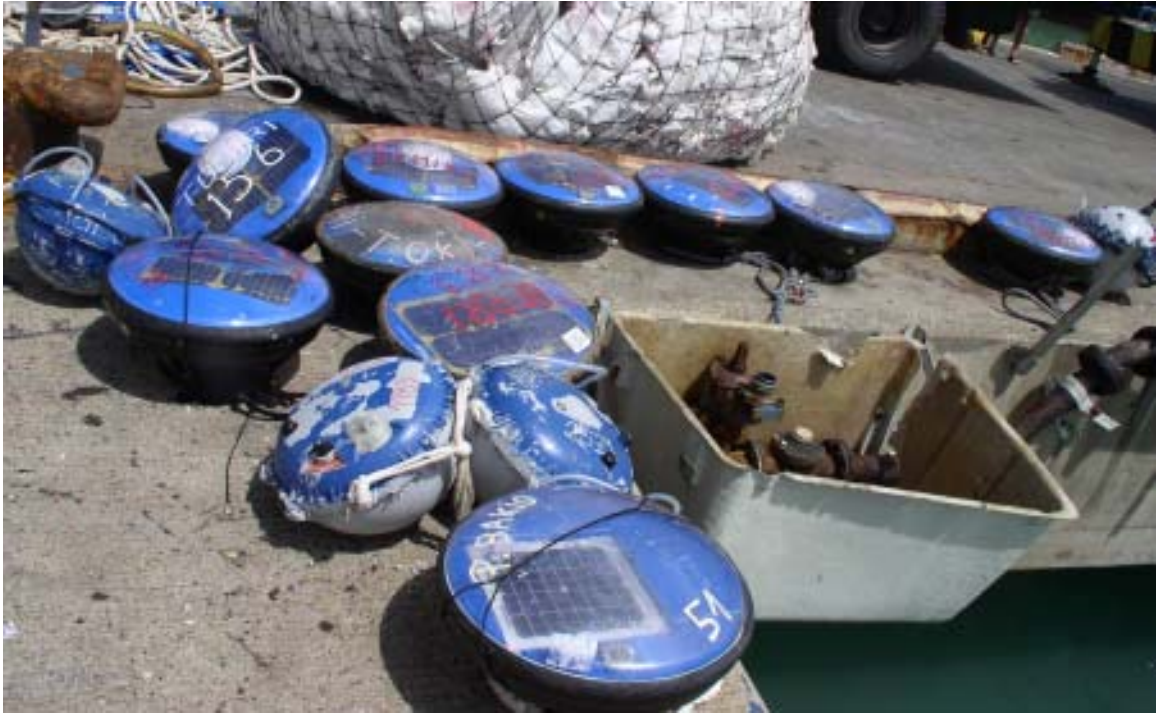
Figure 28. A variety of low profile GPS radio buoys including sonar transmitting units used to mark DFADs (photo Itano)
