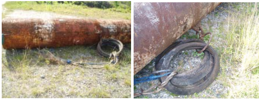
Figure 13. FAD mooring cable attached to FAD swivel with automobile tires
