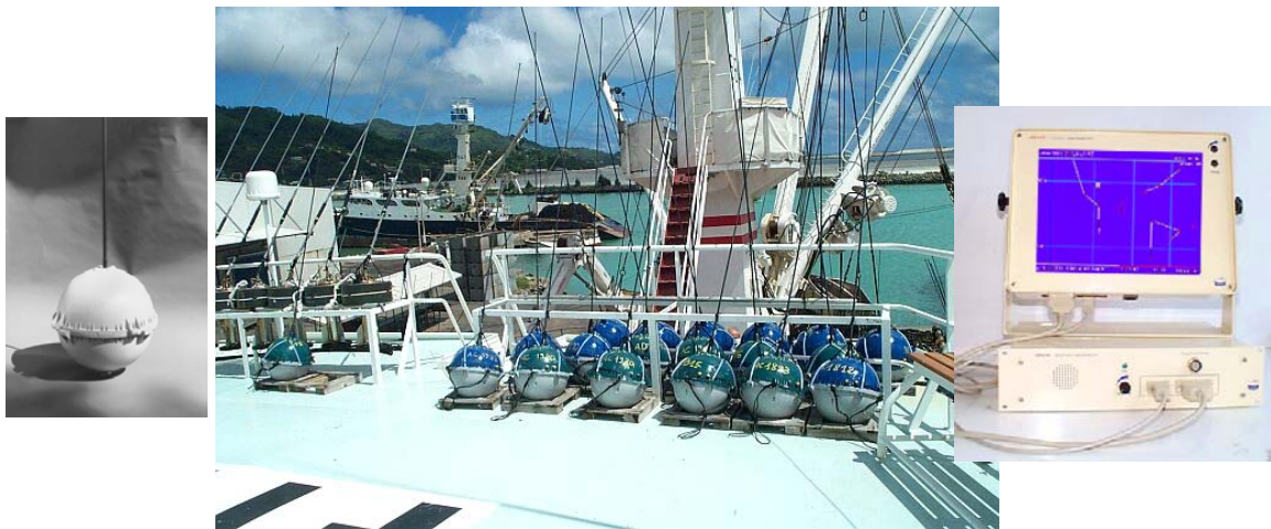
Figure 25. Serpe type GPS tracking radio buoys and computer interface (Martec)
