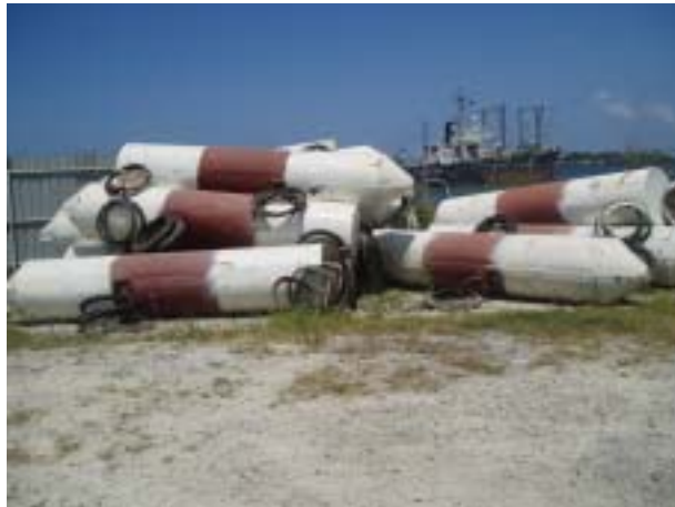
Figure 11. Newly constructed cylindrical steel anchored FAD floats (photos Fukofuka)
