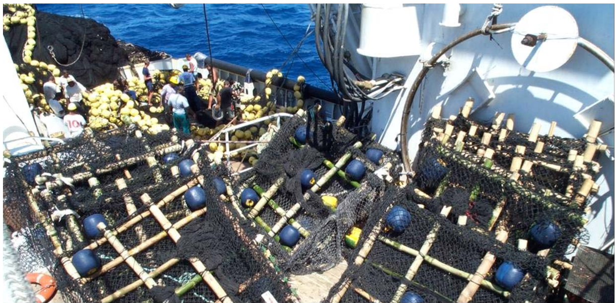
Figure 20. DFADs constructed of bamboo and purse seine netting on the deck of an EU purse seiner in the Indian Ocean (photo Fonteneau)
