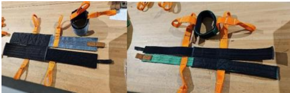
Figure 4. Large (left) and small (right) shark velcros.
