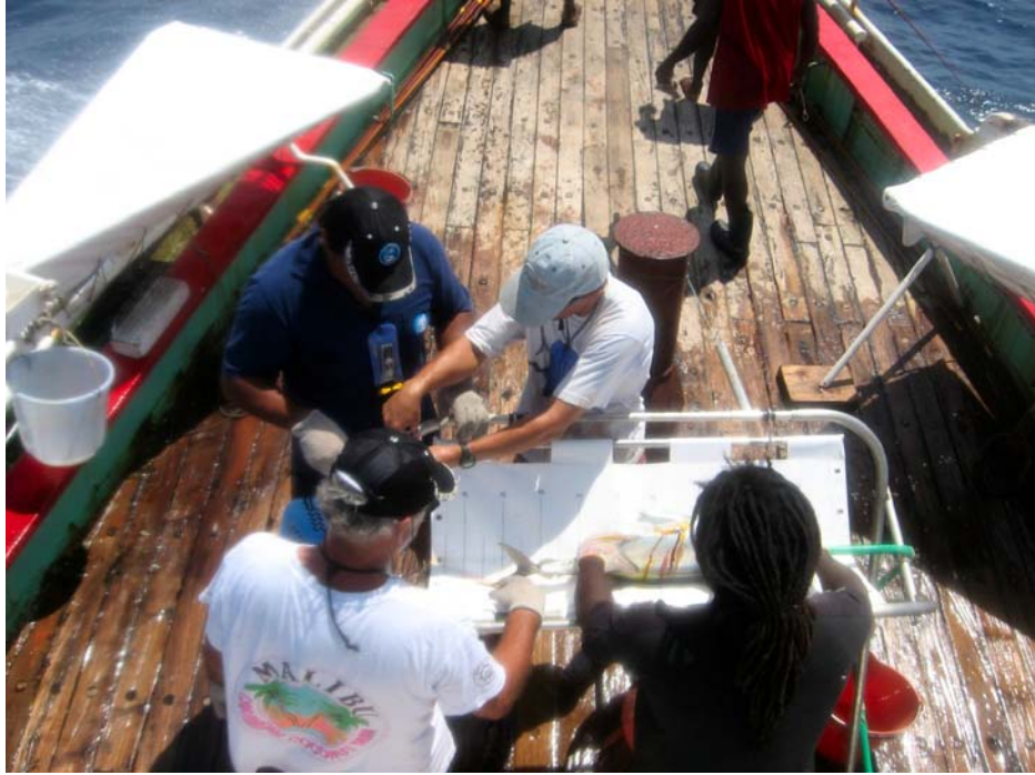
Figure 6. Archival/sonic tagging cradle on the bow
