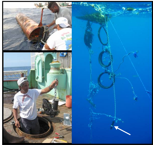
Figure 5. VR2 receiver mounting system.
