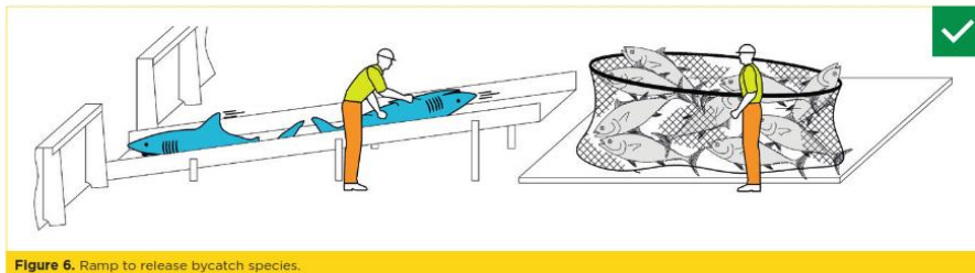
Figure 6. Ramp to release bycatch species.
