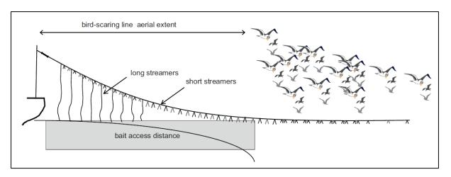
Figure 1. Schematic diagram of a bird-scaring line deployed astern a pelagic longline vessel. (Modified from Melvin et al. 2014).
