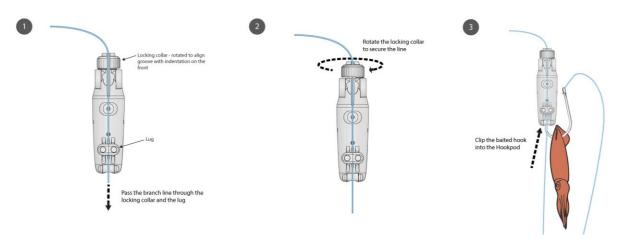
Figure 7. Hookpod attachment to the branchline of a pelagic longline. (Source: B. Ingram, Hookpod Ltd).
