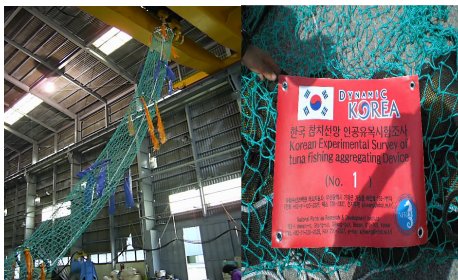
Fig. 2. An experimental FAD with hanging net and rope strands (left), and identification of FAD (right).
