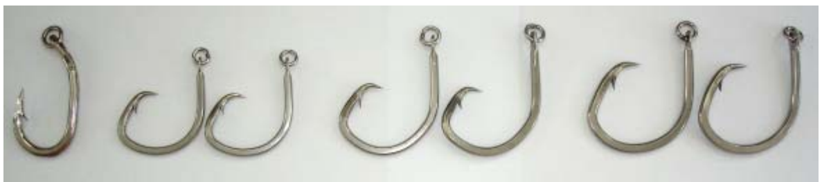
Figure 2. Seven types of longline hooks deployed on the research longline cruise: one size of traditional tuna hook (J 4) with a 5° offset and three sizes of circle hooks (C15o, C15s, C16o, C16s, C18o, C18s) with a 10° offset.
