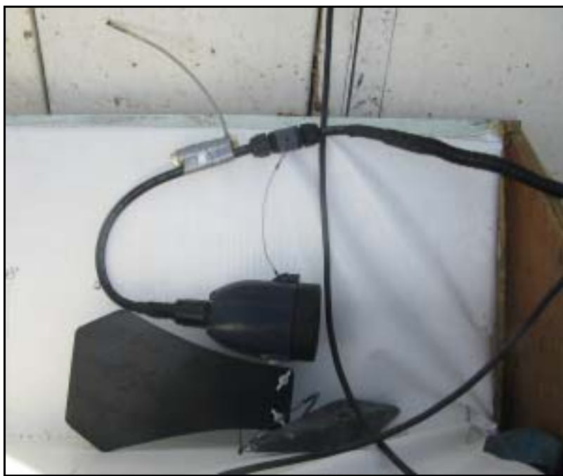
Figure 1. Splashcam Deep Blue color video camera ready to deploy.
