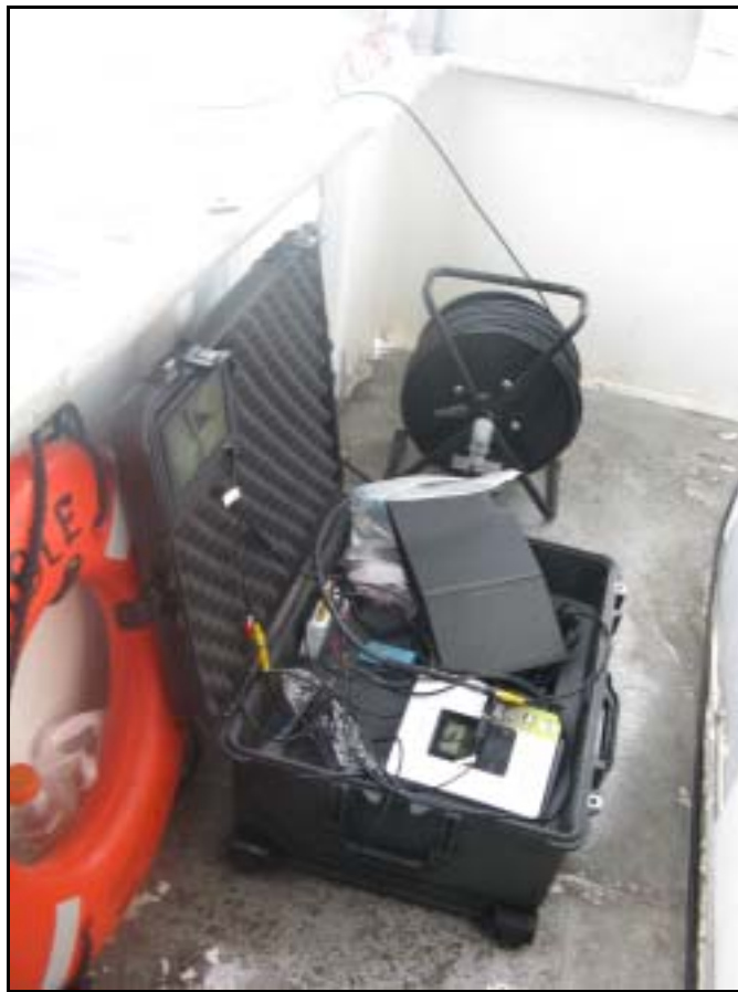
Figure 2. Cable reel, viewing screen and recording components of video system.
