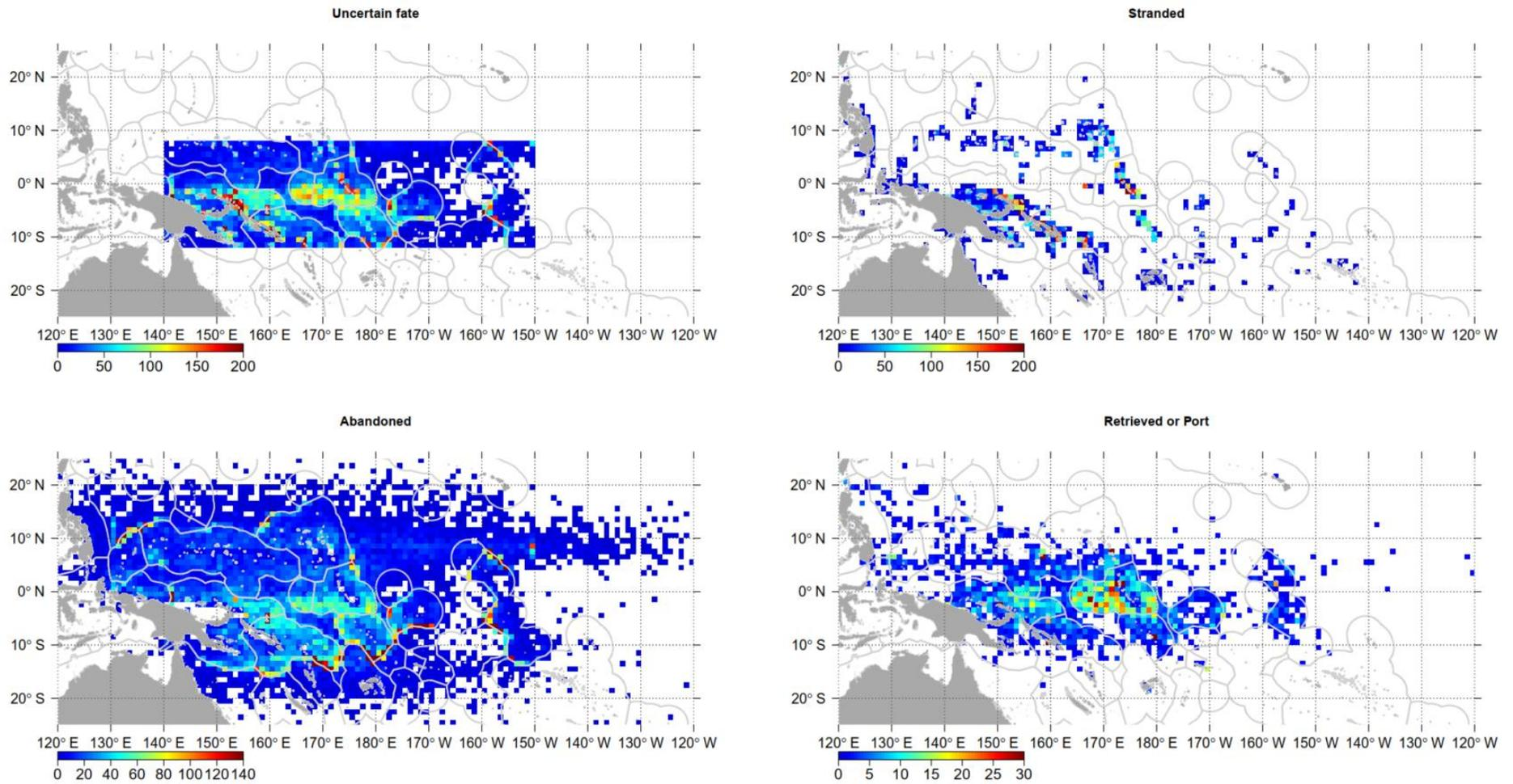
**Figure 16.** Density maps of last recorded position of each buoy in the PNA FAD tracking data: a) uncertain fate; b) stranded; c) abandoned; and d) retrieved or in port; for the 2016–2023 period.
