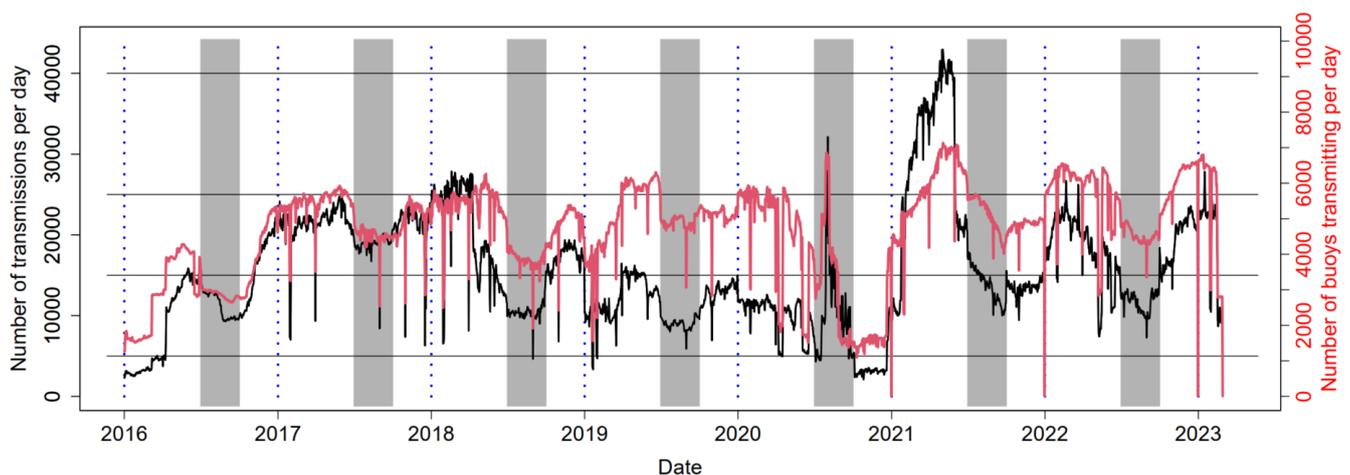
**Figure 7.** Number of transmissions (black line and y-axis 1) and unique buoys transmitting (red line and y-axis 2) daily from at-sea buoy positions only in the PNA FAD tracking dataset. Grey areas correspond to the FAD-closure periods (1<sup>st</sup> of July through 30<sup>th</sup> of September), and the grey dotted vertical denote January 1<sup>st</sup>. Vertical lines indicate levels of 5,000, 10,000 25,000 and 40,000 transmissions.
