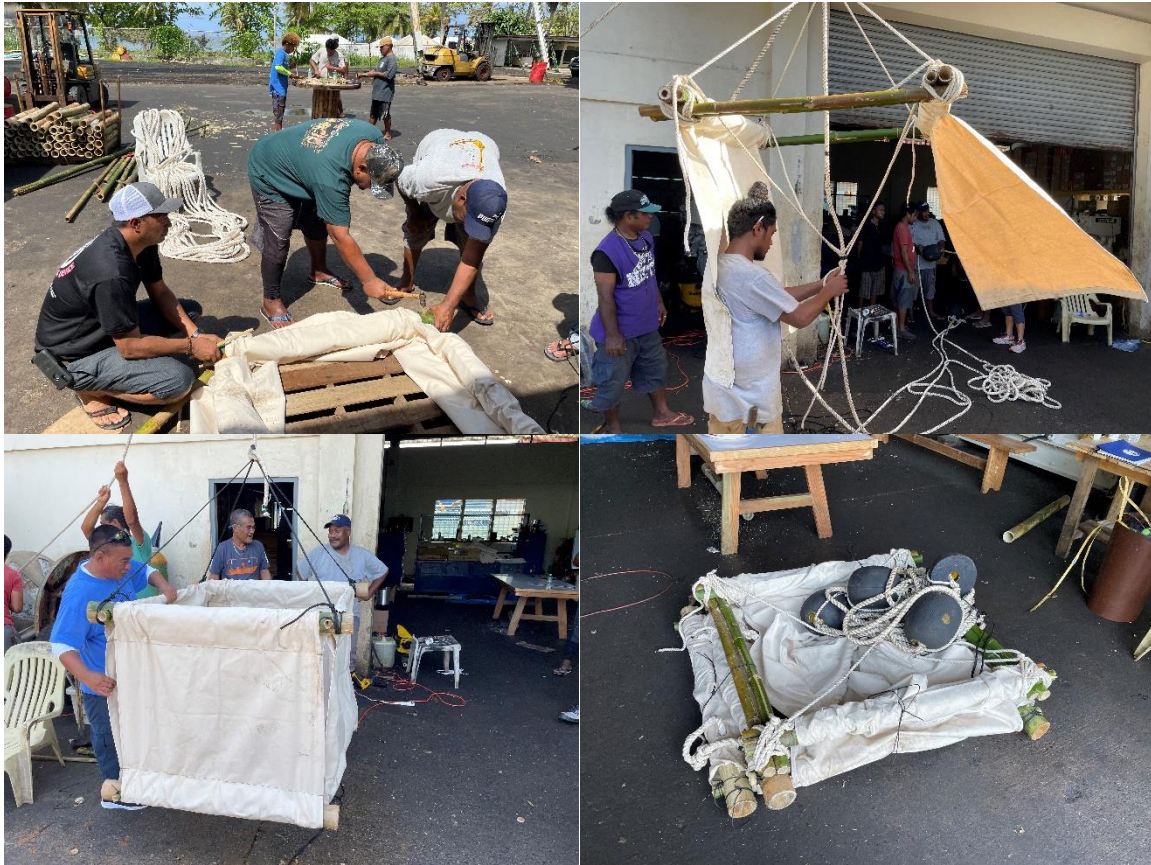
Figure 3. Photos of the construction of the jelly-FADs in Pohnpei.
