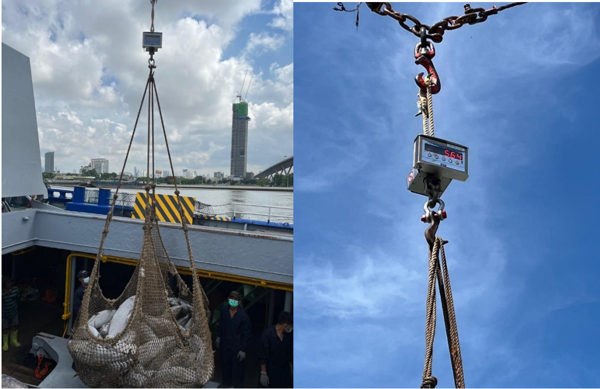
Figure 4. The Phase 2 integrated crane scale undergoing dock side certification/verification testing during offloading activities of the F/V SHC102, Bangkok, Thailand.
