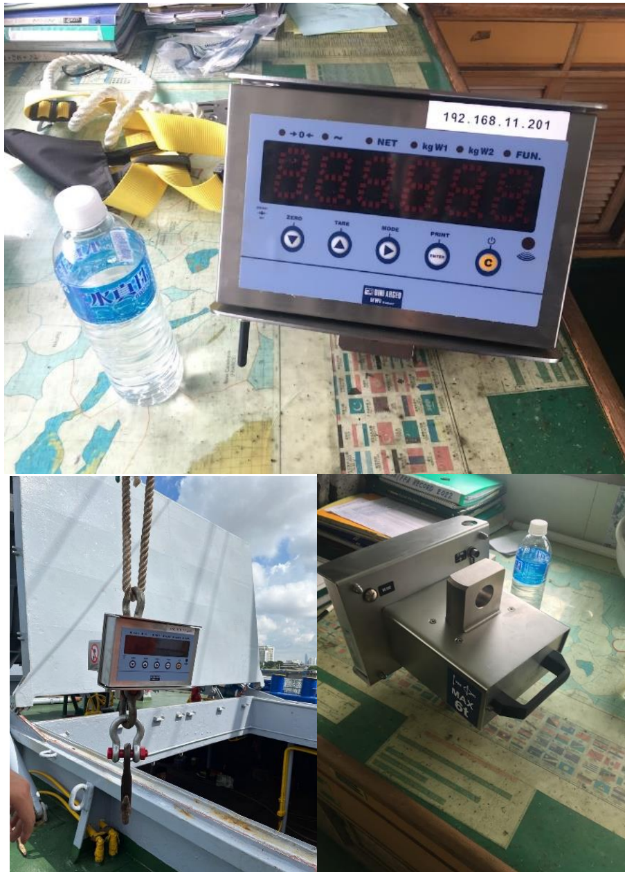
Figure 3. The Italian made DINI ARGEO MCW 09T6-1 5 motion-compensated digital crane scaled used for Phase 2 field work. Specs include a 6 mt capacity, 24-48 hr. rechargeable battery life, and waterproof design (1.5m, 30 min submersion).
