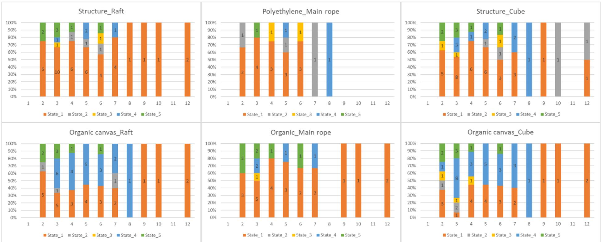
**Figure 10.** Degradation of the different components over time in months (X-axis). State 1 = good condition, State 2 = starting to degrade, 3 = bad state need of repair. State 4 = component not present and State 5 = unknown. Number of observations are written in the columns.
