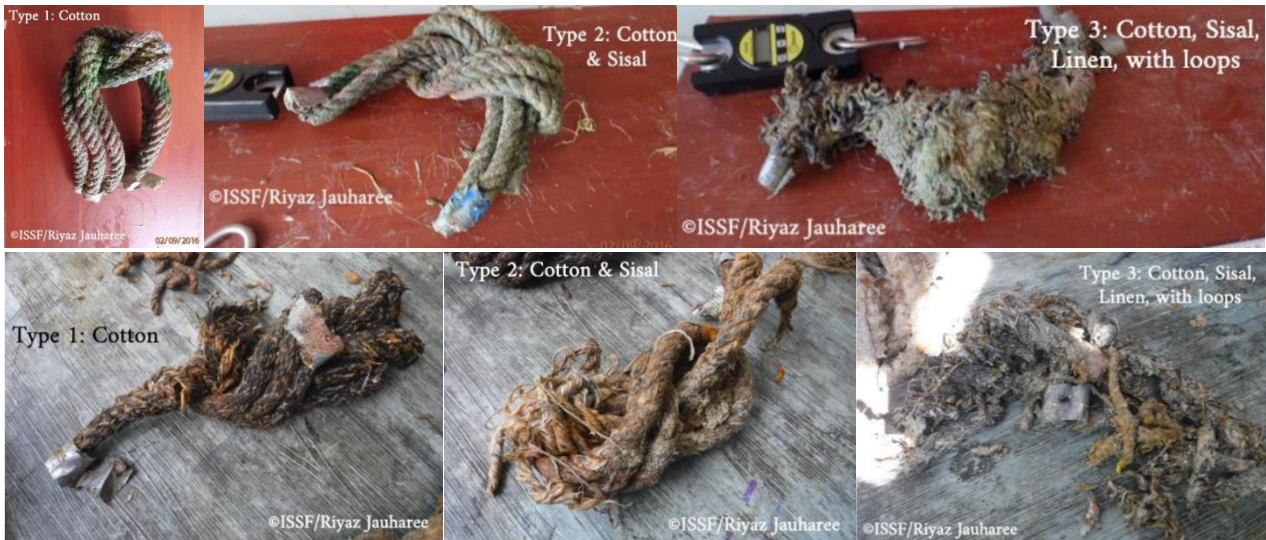
Figure 37. Biodegradable ropes tested by Moreno et al. (2019, 2017b) after 2 (top) and 12 (bottom) months at-sea.
