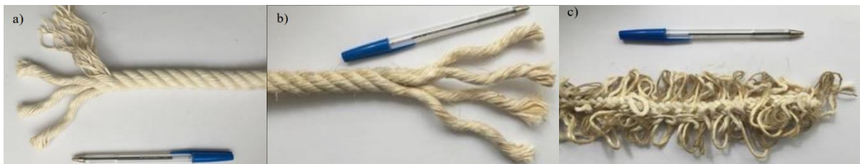
Figure 34. Biodegradable ropes made of (a) 100 % cotton; b) 50% cotton and 50% sisal; and c) cotton, sisal and linen rope with loops, tested by Moreno et al. (2017b).
