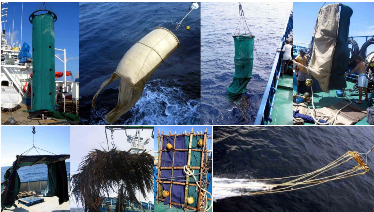
Figure 4. Examples of dFAD designs tested in the scientific trial to reduce entanglement of sharks and turtles from Delgado de Molina et al. (2006).
