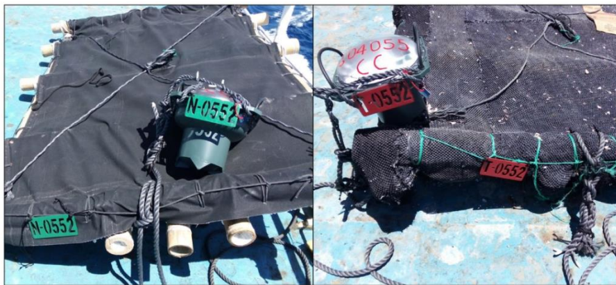
Figure 20. Prototypes of NE BIO dFADs and conventional dFAD tested in the EPO, with corresponding marking (Román et al., 2022, 2020).
