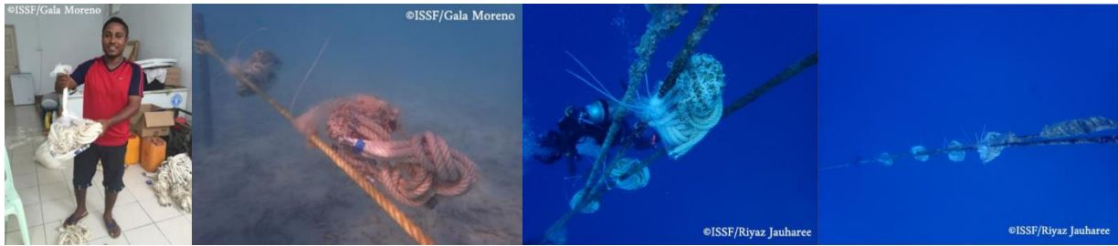
Figure 36. Settings of the experiment to study degradation with time of biodegradable ropes in Maldives, tested by Moreno et al. (2019, 2017b).
