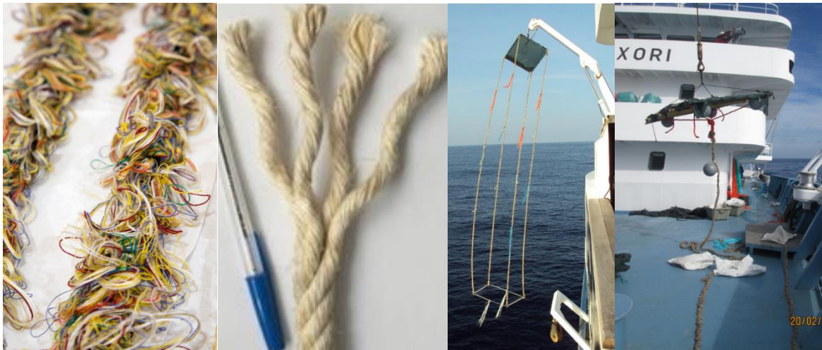
Figure 13. Biodegradable ropes made of 100 % cotton without loop (left) and 100 % cotton with loops (center left), used to construct biodegradable dFAD tested in real fishing conditions in the IO by Moreno et al. (2017c). Two designs were tested, a shallower dFAD at 10 m and 30 m depth (Center right); and d) a deeper dFAD at depths of 30 m, 50 m and 70 m.
