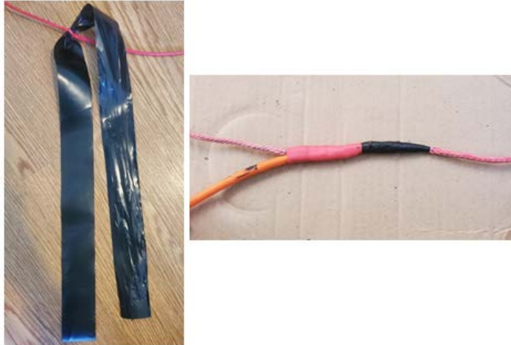
Figure 2. Pictures showing how each streamer type was attached to the tori line backbone. Black short streamers fed in through the hollow 3 mm red dyneema backbone, and the rubber tubing lashed on and then sealed with pink marine grade shrink wrap attached to the aerial extent backbone via heat gun, and then wrapped with electric tape to prevent possible snags at the edges.
