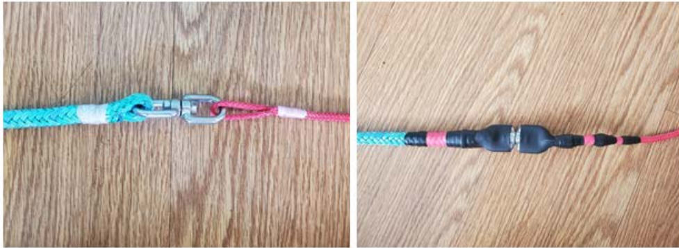
Figure 4. The two-step process taken to join the aerial and drag components. Step 1 consisted of creating the joints via swivel and eye splice, and step 2 involved sealing the joint with shrink wrap, a heat gun, and electrical tape to minimize the possibility of snagging.
