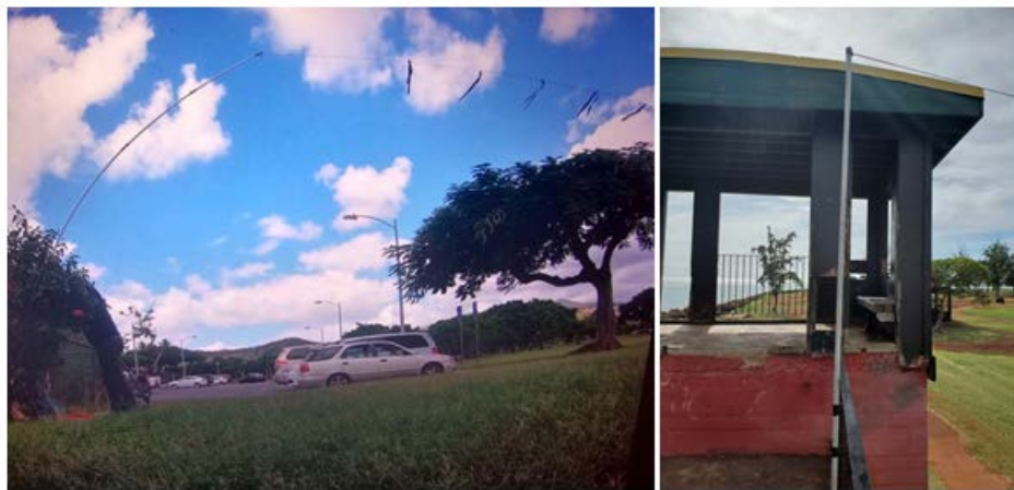
Figure 5. Fiberglass tori pole flexing with the 60 m short streamer line (left), and 316 Sch.40 marine grade Steel pole flexing with the 60 m short streamer line (right).
