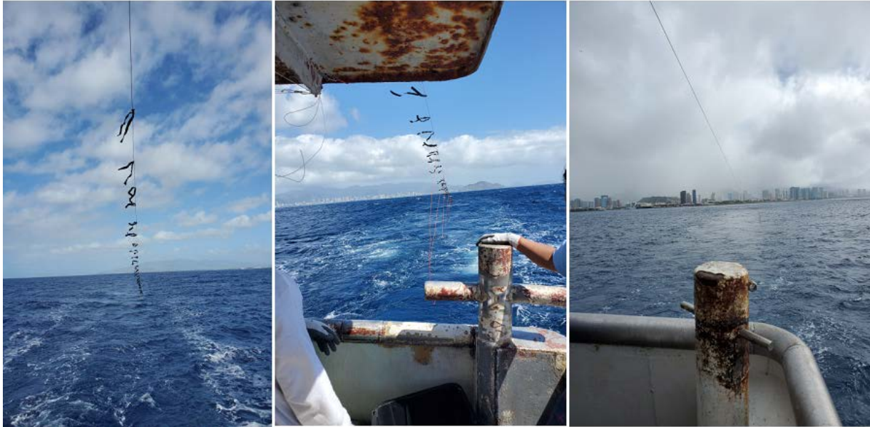
Figure 11. 105 m short streamer line being flown; 165 m hybrid streamer line being flown; 105 m streamerless design being flown during Phase 1 demonstration trips with no fishing gear deployed.
